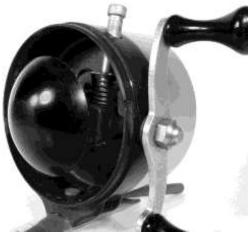
The back cover of this first Zebco reel has been removed to show Hull's clutch, the subject of his January, 1949, patent application. The plastic dome, or "disc," prevents spool rotation when pressed by the angler's thumb.
