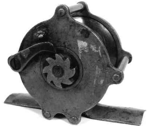
A riveted brass multiplier with an anti-reverse pawl-and-ratchet.
