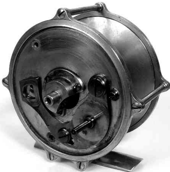
Kopf's clutch in a German silver/hard rubber reel. A pin extends into the hole at the end of the curved plate and swivels the plate when it is shifted by a lever. The reel is significantly larger than the Mills "Imperial" bass reels and is suitable for saltwater fishing.
