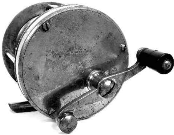
A typical New York-style, brass reel marked with Kopf's name. Note that the crank is a reverse "S".
