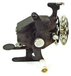
Sawitzke's "Taffy" reel. The spool spins freely unless the thumb lever is depressed to engage the friction clutch. The line goes through the agate guide above the spool. The knurled screw just behind the spool is an anti-backlash device, which would not be needed for a fixed-spool reel.
