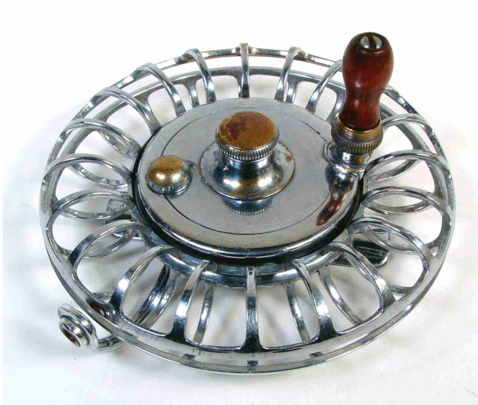
The Sellers side-mounted fly reel, made of plated brass. The “spokes” taper slightly and are wider at the distal ends. Loosening the knurled nut at its base allows the handle to be folded down.
