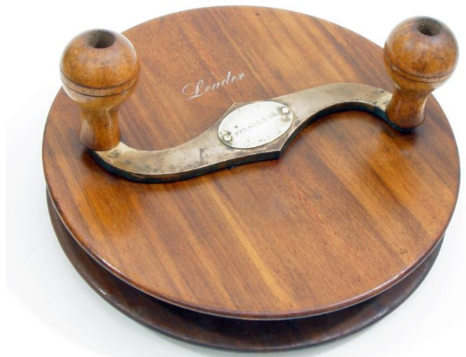
A wooden "Leader" side-mounted reel with Smith's patent date stamped on the central plaque. The spool has a flat arbor and uses ball bearings in flat-sided races.
