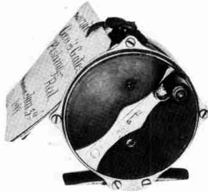
Gates' reel, showing the sliding spring which frees the driveshaft from the crank to permit the operation of the drag.
