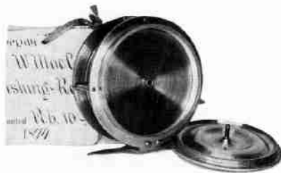
MacCord's spool can be removed after the rear cover is unscrewed. The spool is driven by a four-gear train operated by a crank mounted at the center of the front cover.
