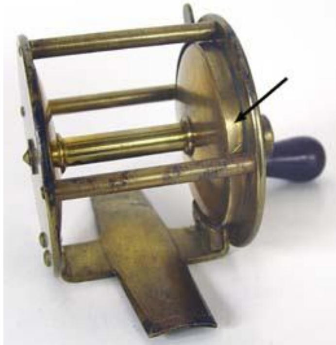
This view of the larger early reel shows the sheet-metal foot and the circular flange that forms the gear box (arrow). The foot is attached by two rivets and a screw, which enters a supporting block. Such blocks were often used with the patented foot.
