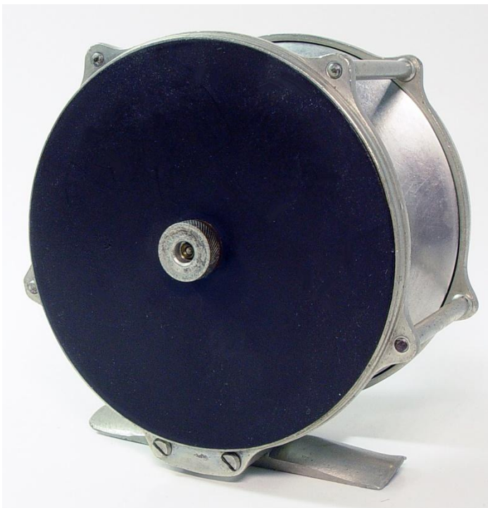
Tailplate of the Gates reel. The knurled nut adjusts the tension on the interior spring and, thereby, on the drag shoe.
