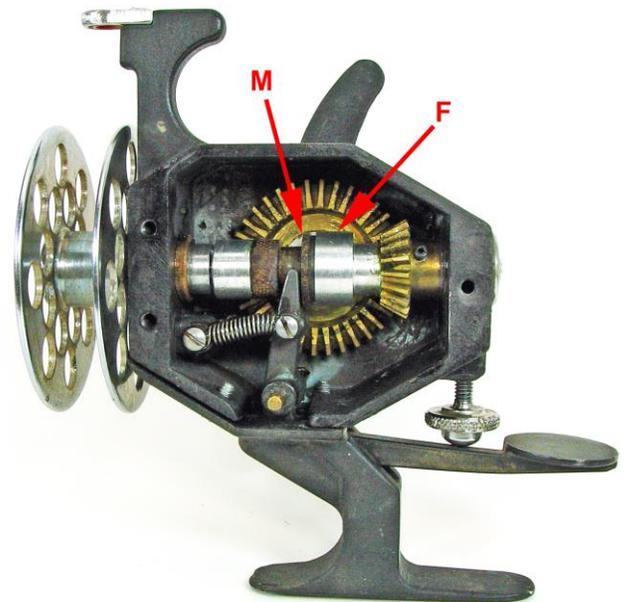
*The pressure between the male (M) and female (F) members of the friction clutch is adjusted by the thumb lever. The clutch members are made of Micarta and aluminum, respectively. The knurled screw above the lever can hold the lever at a pre-selected position.*
